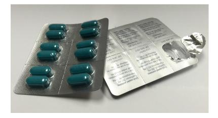
Hard tempered foil is more rigid and can be punctured without compromising its overall strength. It is ideal for blister packs as shown here.
