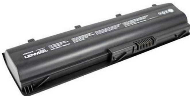
Typical laptop battery, containing multiple lithium-ion cells
